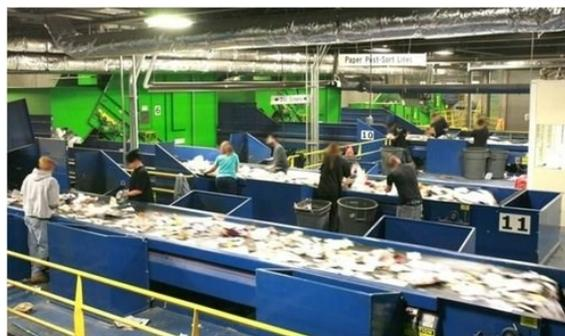
There, the materials are loaded onto conveyor belts where employees in pre-sort lines manually remove large metal, plastic or paper items as well as anything that might be harmful including plastic bags, sharps, rope and trash. Glass is removed early in the process to prevent damage to the conveyor belts and equipment.
